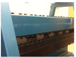
measurement system of and the results are specific to CSU's magnet. An aspect making this project unique is that it will take into account dispersion of the resulting frequency components within the wire thereby making the measurement much more accurate. The undulator will eventually be a key part of the accelerator system in creating light. The goal is to get smooth magnetic field transitions between the dipoles throughout the undulator.
